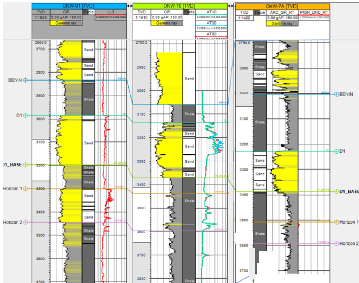
Figure 5: Well logs showing Gamma, lithofacies and Resistivity Logs
