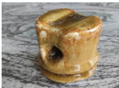
Plate 2: Glaze-fired porcelain insulator with smooth glassy surface
