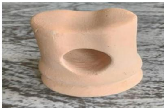
Plate 1: Bisque-fired porcelain insulator prototype
