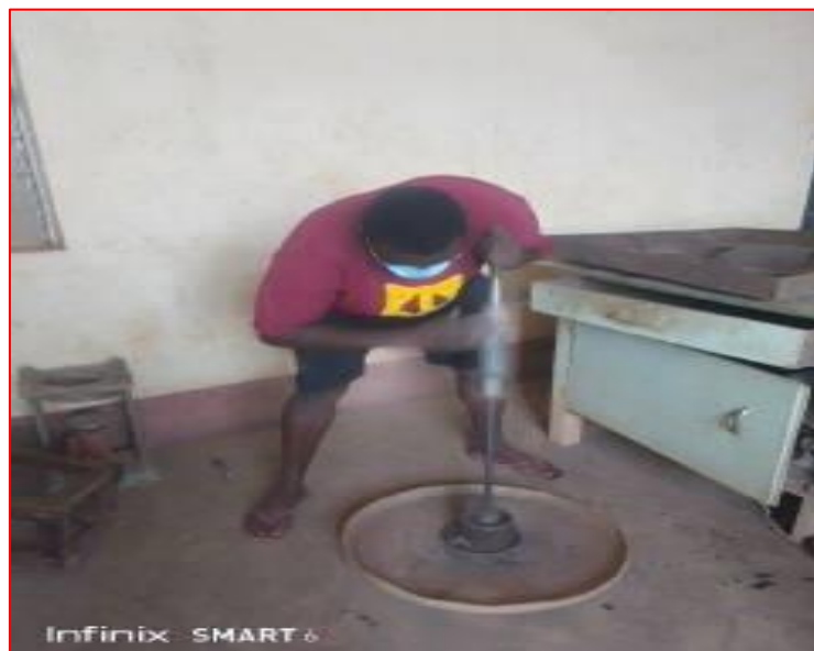
Figure 7: Showing lab procedure of compaction test
