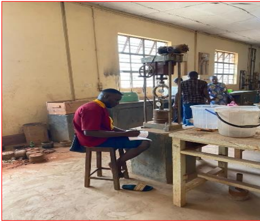
Figure 8: Showing laboratory procedures for California Bearing Ratio test
