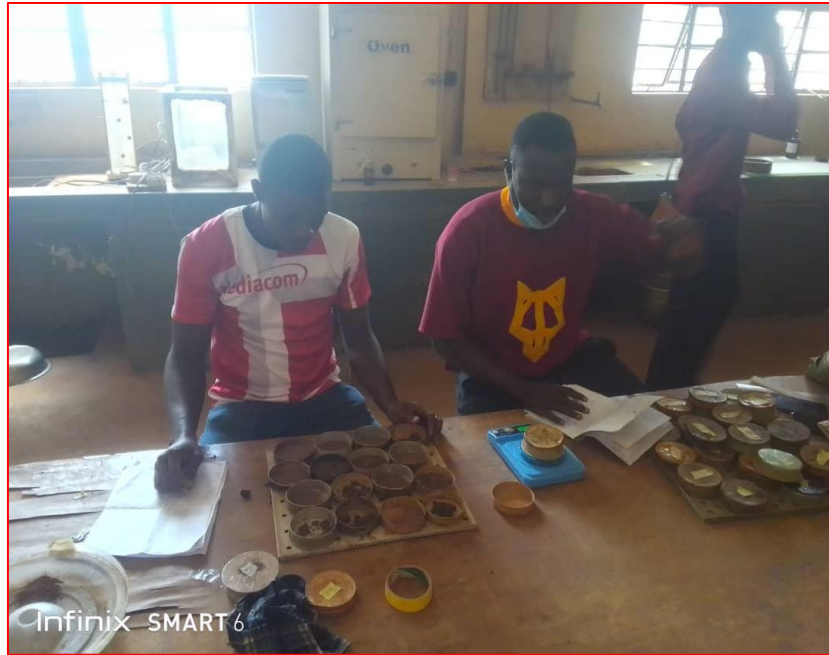
Figure 4: Showing lab procedures of moisture content
