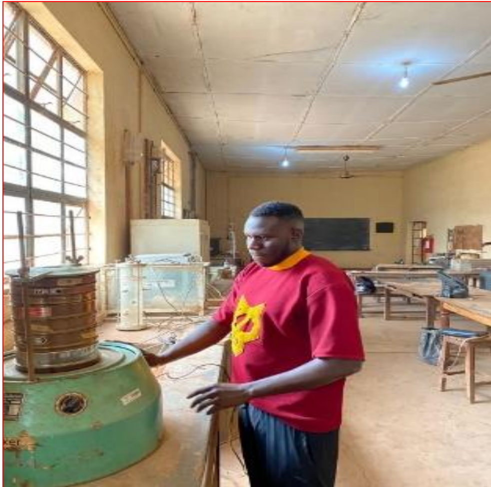
Figure 3. Showing lab procedures of particle size analysis
